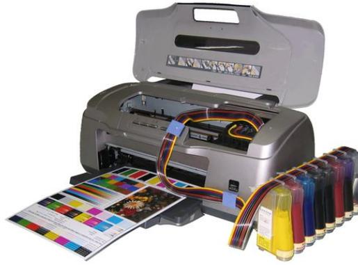
Figure 2.3: Continuous Ink Supply System (CISS)
